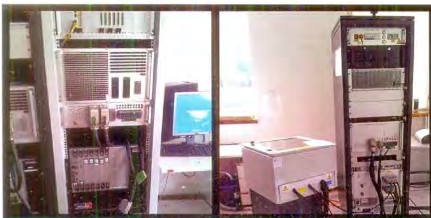
Alten has 20 Hardware-In-the-Loop (HIL) test benches in Europe to validate powertrain and electronic systems. It plans to transfer tech and expertise to its auto testing facility in Chennai.
